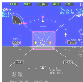
Fig. 16 Core modes — Altitude select/hold example.
